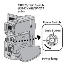
When the Power Switch is set to " ▲ ", " ▲ " appears. When set to " M " or " ℡▲ ", there is no indication.
