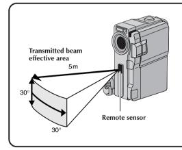
When using the remote control, be sure to point it at the remote sensor. The illustration shows the approximate transmitted beam effective area for indoor use.
