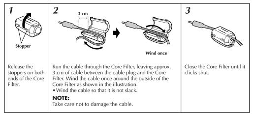
When connecting cables, attach the end with the Core Filter to the camcorder.
